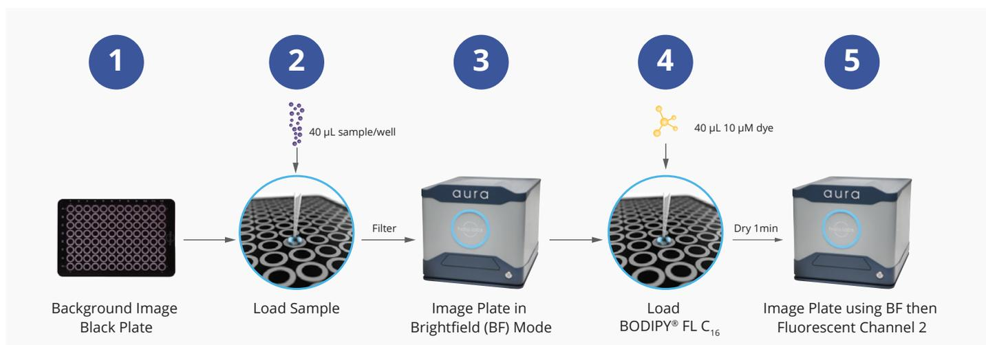
**Figure 1:** The polysorbate degradation assay workflow on the Aura detects degraded excipients, even in high concentration protein formulations. Samples are labeled with Thioflavin-T and BODIPY FL C<sub>16</sub> to specifically ID protein aggregates and free fatty acids, respectively, with FMM.
